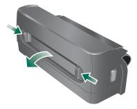
**d** Reinsert the rear access panel or the auto-duplex unit into the printer.
