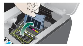
5 Lift the handle of a printhead and use it to pull the printhead out of its slot.
