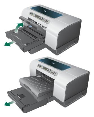
If you are loading A3 or larger sized media, extend the tray by pressing the tray extension lock near the front of the tray and pulling both ends of the tray in opposite directions until it is fully extended.
