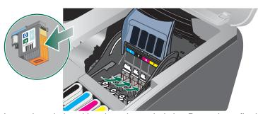
Insert the printhead into its color-coded slot. Press down firmly on the printhead to ensure proper contact.
