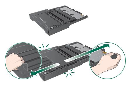
Press the button of the media width guide and slide the guide to the left. Press the button of the media length guide and slide the guide towards you.
