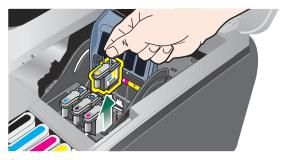
Carefully remove any ink from the contact pads on the printhead using a dry cotton swab or a soft, dry, lint-free cloth that will not come apart or leave fibers behind.
