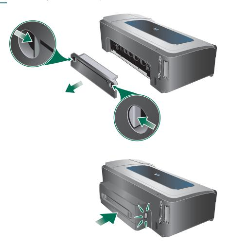
Enable the auto-duplex unit in the printer driver. See Enabling accessories in the printer driver.
