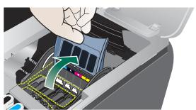
Lift the handle of a printhead and use it to pull the printhead out of its slot.
