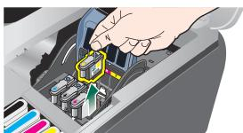
Remove the new printhead from its package, and then remove the protective tape. 5
