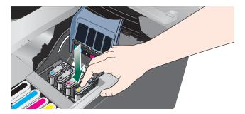
7 Close the printhead latch. Press down to ensure it is in the lock position.
