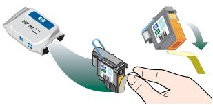
Insert the printhead into its color-coded slot. Press down firmly on the printhead to ensure proper contact.
