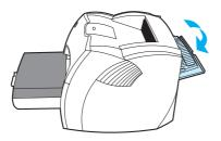
**2** Before loading the envelopes, slide the media guides outward to slightly wider than the envelopes.
