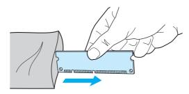
**5** Position the DIMM chip in front of the slot located inside the I/O door. The gold contacts should be pointing toward the printer and the cutouts should be at the top and bottom.
