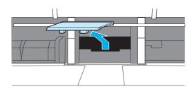
6 With one hand, position the new separation pad in the slot of the previous separation pad (A). With the other hand, reach through the input tray opening, and push the spring-loaded base down (B).
