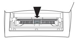
4 To pry the separation pad up from the spring-loaded base, insert a flat-edged screwdriver in the slot under the separation pad and twist until the tabs are free.
