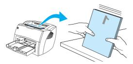
8 Place the stack back in the input tray. Side one should be facing down with the bottom edge feeding into the printer first. Replace the priority input tray.
