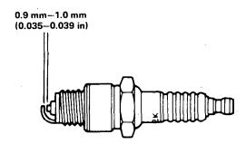
5. Attach the plug washer. Thread the plug in by hand to prevent cross-threading.
