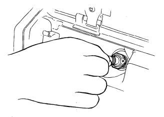
6. Tighten a new spark plug 1/2 turn with the wrench to compress the washer. If you are reusing a plug, it should only take 1/8–1/4 turn after the plug seats.
