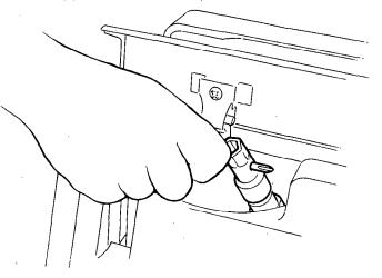
3. Visually inspect the spark plug. Discard it if the insulator is cracked or chipped. Clean the spark plug with a wire brush if it is to be reused.
