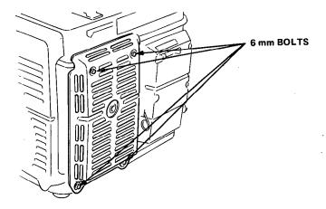
2. Remove the two 6 mm nuts and the 6 mm bolt. Remove the muffler from the exhaust pipe carefully to avoid damaging the spark arrester screen.
