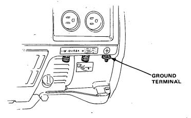
NOTE: The EX800 generates both AC and DC power. If you use both at the same time, be sure not to exceed the total rated power of 700 W for AC and DC.
