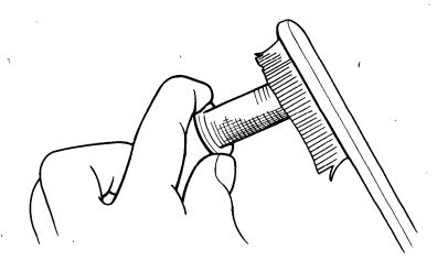
4. Check the exhaust pipe gaskets; replace if damaged. Reinstall the muffler and the cover.
