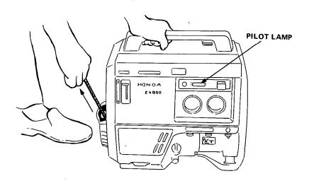
CAUTION: Do not allow the starter grip to snap back against the generator. Return it gently to prevent damage to the housing.
