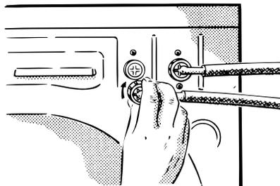
2. Connect the straight end of the hoses to the stop taps.
