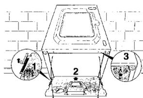
**Note: we recommend you keep the transit bracket and screws to protect the machine for future transit. The Manufacturers will not be responsible for any damage to the machine caused by not following the instructions relating to releasing the transit protection. The user is responsible for all installation costs.**
