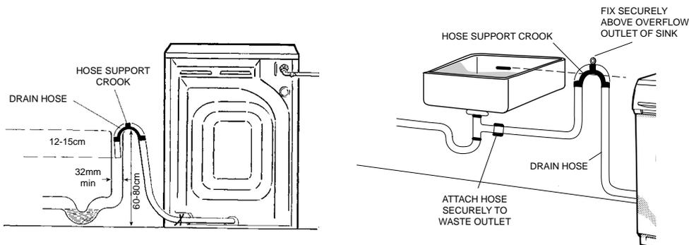
**For the washing machine to function properly the outlet end of the drain hose must be at a minimum of 60 cm and a maximum of 80 cm from the ground.**
