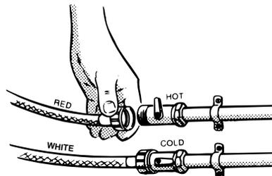
If the inlet hose's connection point is changed, check that the 3/4" threaded ferrule on the inlet hose is firmly attached to the electrovalve connector.
