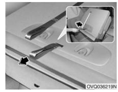
3. Pull the seat by using the stowing strap.
