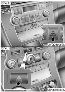
The hazard warning flasher causes the front and rear turn signal lights to flash on and off, which serves as a warning to other drivers to exercise caution when approaching or passing your vehicle.
