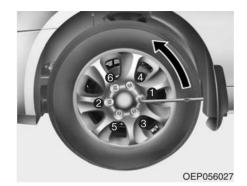
Loosen the wheel lug nuts counterclockwise one turn each, but do not remove any nut until the tire has been raised off the ground.
