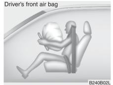
Upon deployment, tear seams molded directly into the pad covers will separate under pressure from the expansion of the air bags. Further opening of the covers then allows full inflation of the air bags.
