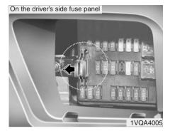
How to reset the power sliding door and power tailgate
