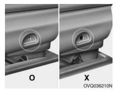
4. Make sure the green mark on the rear seat cushion frame is visible and the catches are locked in position by moving the seat forward and backward or lifting the front portion of the seat. If the green mark is not visible and the seat moves, it is not locked properly.
