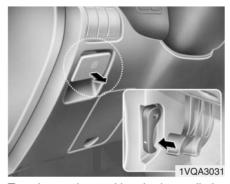
To release the parking brake, pull the parking brake release lever while applying the service brake. The pedal will automatically extend to the fully released position. If the parking brake pedal does not release or does not release all the way, have the system checked by an authorized Hyundai dealer.
