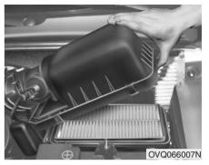
2. Wipe the inside of the air cleaner housing with a clean, damp cloth.
