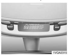
The trip computer is a microcomputercontrolled driver information system that displays information related to driving, including compass, distance to empty, driving time, average fuel consumption and outside temperature on the display when the ignition switch is in the ON position. All stored driving information is reset if the battery is disconnected.
