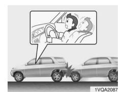
Frontal air bags are not designed to inflate in rear collisions, because occupants are moved backward by the force of the impact. In this case, inflated air bags would not be able to provide any additional benefit.
