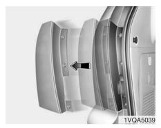
3. Remove the rear combination light assembly from the body of the vehicle.
