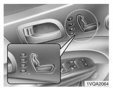
A driver position memory system is provided to store and recall the driver seat, outside rearview mirror and adjustable pedal positions with a simple button operation. By saving the desired positions into the system memory, different drivers can reposition the driver seat, outside rearview mirror and adjustable pedals based upon their driving preference.
