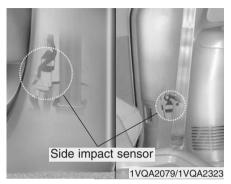
The side impact air bags are designed to deploy only during certain side-impact collisions, depending on the crash severity, angle, speed and point of impact. The side impact air bags are not designed to deploy in all side impact situations.
