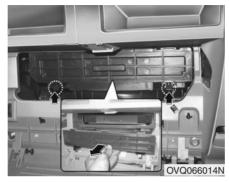
3. Remove the climate control air filter cover pulling up both taps of the cover.
