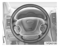
To sound the horn, press the area indicated by the horn symbol on your steering wheel (see illustration). The horn will operate only when this area is pressed. Check the horn regularly to be sure it operates properly.
