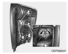
Remove the socket from the assembly by turning the socket counterclockwise until the tabs on the socket align with the slots on the assembly.
