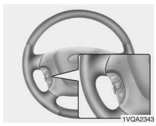
Remote audio control buttons are provided on the steering wheel.
