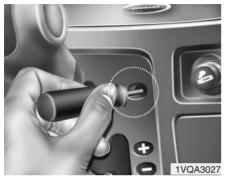
Insert a screwdriver into the access hole and press down on the screwdriver.
