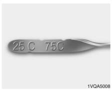
If the fluid has been warmed to normal operating temperature of approximately 158~176°F (70~80°C), the fluid level should be within "HOT" range.
