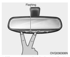
When programming the buttons for the first time, press and hold the left and center buttons ( 1, 1) simultaneously until the indicator light begins to flash after approximately 20 seconds. (This procedure erases the factory-set default codes. Do not perform this step to program additional hand-held transmitters.)
