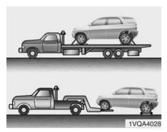
If emergency towing is necessary, we recommend having it done by an authorized Hyundai dealer or a commercial tow-truck service. Proper lifting and towing procedures are necessary to prevent damage to the vehicle. The use of wheel dollies or flatbed is recommended.
