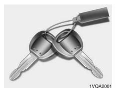
The key code number is stamped on the plate attached to the key set. Should you lose your keys, this number will enable an authorized Hyundai Dealer to duplicate the keys easily. Remove the plate and store it in a safe place. Also, record the code number and keep it in a safe and handy place, but not in the vehicle.
