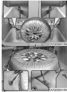
3. Pass one end of the strap through the wheel center and connect both strap hooks to each striker of the 3rd row seat on the floor.
