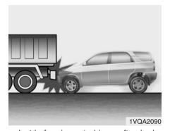
· Just before impact, drivers often brake heavily. Such heavy braking lowers the front portion of the vehicle causing it to "ride" under a vehicle with a higher ground clearance. Air bags may not inflate in this "under-ride" situation because deceleration forces that are detected by sensors may be significantly replaced by such "under-ride" collisions.
