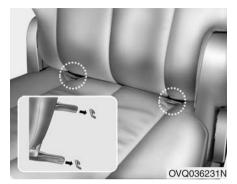
ISOFIX anchors have been provided in your vehicle. The ISOFIX anchors are located in the left and right outboard rear seating positions. Their locations are shown in the illustration. There is no ISOFIX anchor provided for the center rear seating position.
