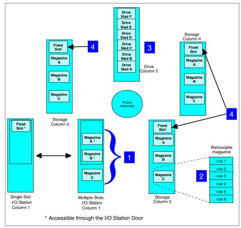
Figure 7-3 IBM 3583-L72 location logical view
