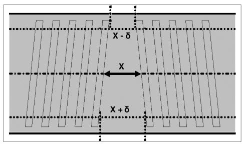
Figure 2-2 Magnified servo band showing a pair of servo bursts
