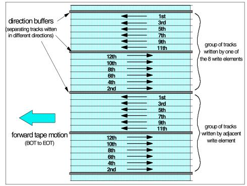
Figure 2-5 Portion of data band showing Ultrium 1 track-writing sequence
