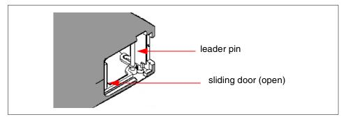
Figure 2-9 Leader pin attached to the tape medium
