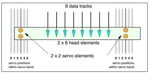
Figure 2-15 Eight-element head (one set of heads shown) and servo elements
