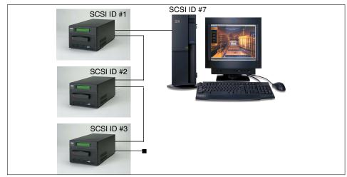
Figure 4-2 SCSI ID set-up example
