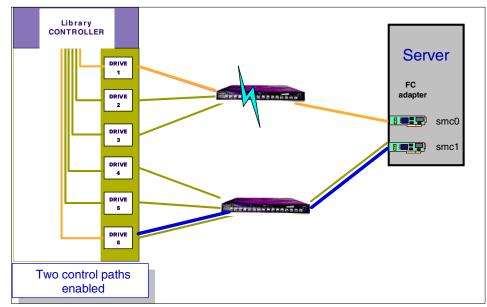
Figure 8-16 Redundant control paths to the library controller
