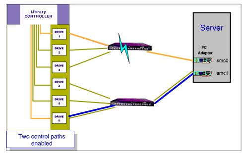
Figure 2-28 Redundant control paths to the library controller
