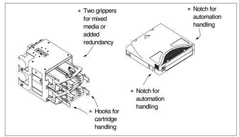
Figure 8-14 IBM 3584 Gripper
