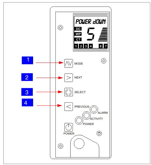
Figure 5-5 IBM 3581 operator panel
