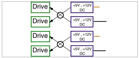
Figure 8-7 Redundant drive power supply
