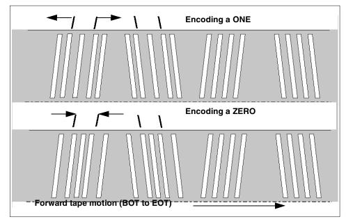
Figure 2-3 Encoding bits using the servo stripes within the servo bursts
