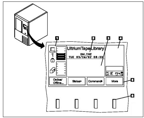
Figure 7-5 IBM 3583 tape library operator panel
