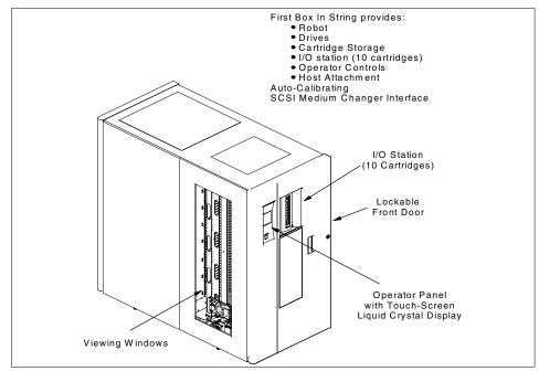
Figure 8-2 IBM 3584-L32 base frame view from front left
