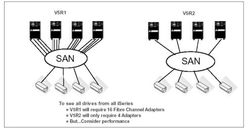
Figure 10-1 Multiple-target support
