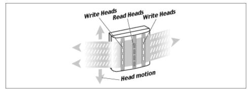
Figure 3-10 DLT 7000/8000 tape head
