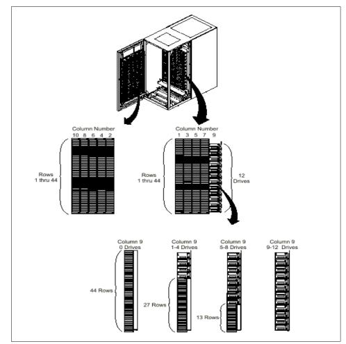
Figure 8-18 IBM 3584-D32 expansion frame showing slot components
