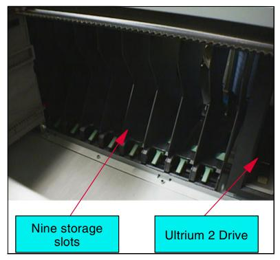
Figure 6-3 IBM 3582 rear-mounted storage slots
