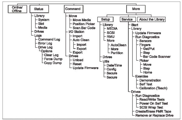
Figure 7-6 IBM 3583 flowchart of library functions
