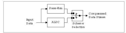
Figure 2-6 LTO-DC block diagram
