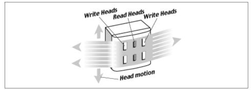
Figure 3-7 DLT 2000 recording head design
