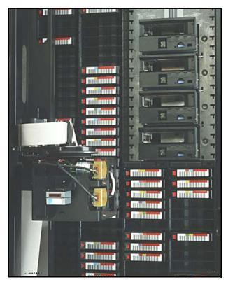
Figure 8-13 IBM 3584 accessor assembly
