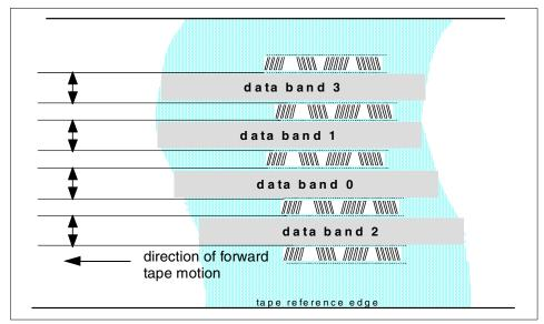
Figure 2-4 Four data bands written between the servo tracks
