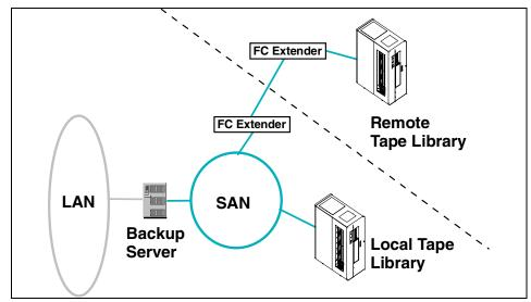
Figure 3-17 Electronic vaulting
