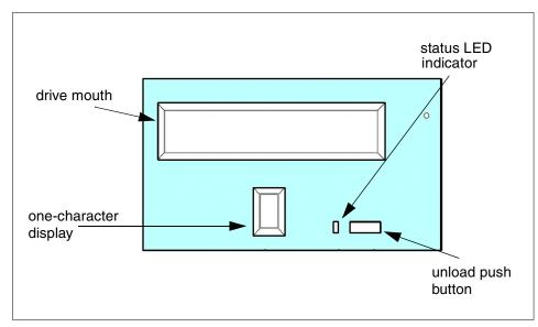
Figure 2-22 Front of subassembly showing operator panel indicators
