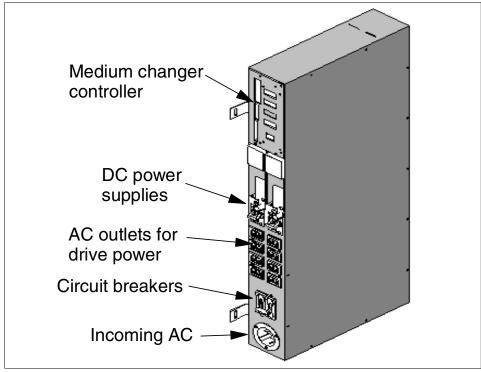
Figure 8-11 Frame controller assembly
