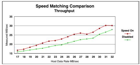
Figure 2-20 Speed matching comparison: MB/sec
