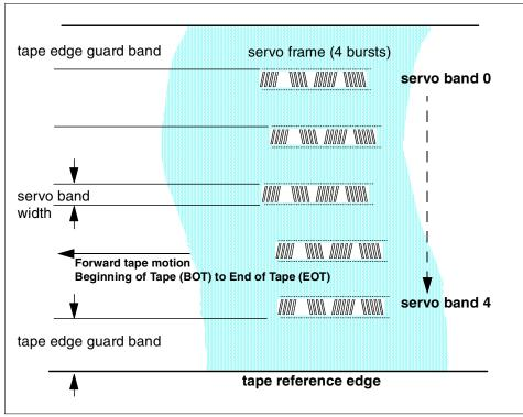
Figure 2-1 Servo band position and nomenclature
