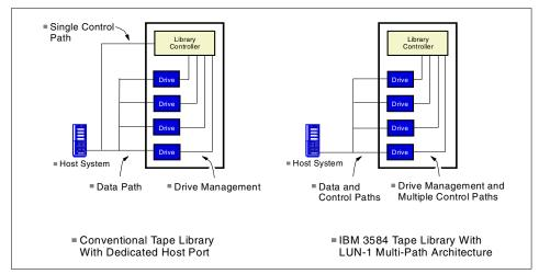
Figure 2-27 Conventional tape library vs. multi-path architecture
