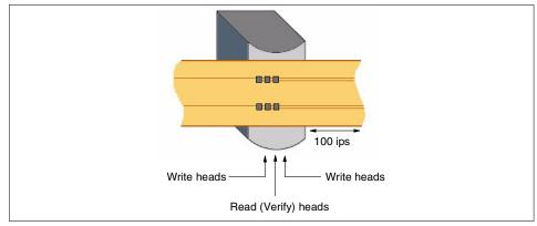
Figure 3-3 QIC head diagram
