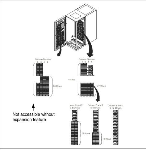
Figure 8-17 IBM 3584-L32 base frame showing cartridge slot components
