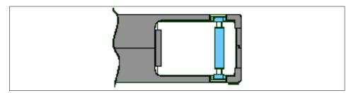
Figure 2-13 Correct leader pin placement
