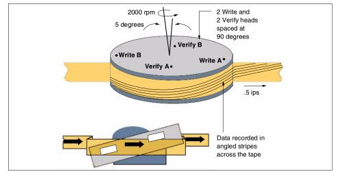
Figure 3-4 Helical-scan recording diagram
