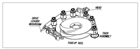
Figure 3-6 DLT tape path mechanism
