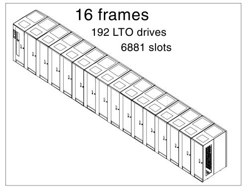
Figure 8-4 IBM 3584 with 16 frames
