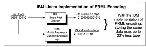
Figure 2-19 IBM linear implementation of PRML encoding
