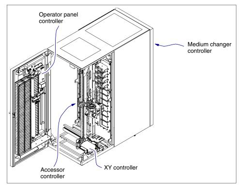
Figure 8-9 IBM 3584 distributed control system
