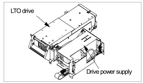
Figure 8-6 IBM 3584 LTO Ultrium tape drive assembly
