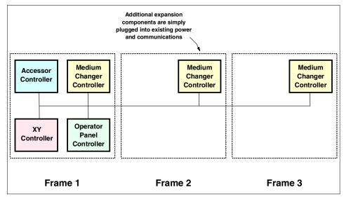
Figure 8-10 Redundant medium changer controller
