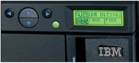
Figure 6-4 IBM 3582 operator panel
