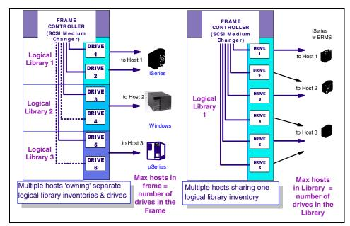
Figure 3-16 IBM 3584 multi-path architecture
