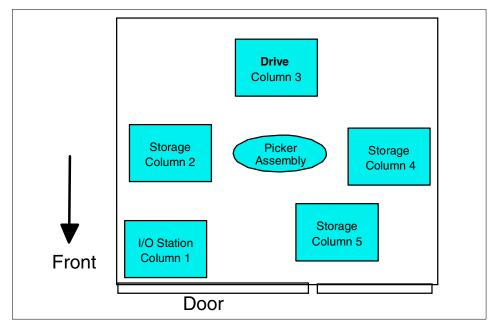
Figure 7-2 IBM 3583 storage columns: top view
