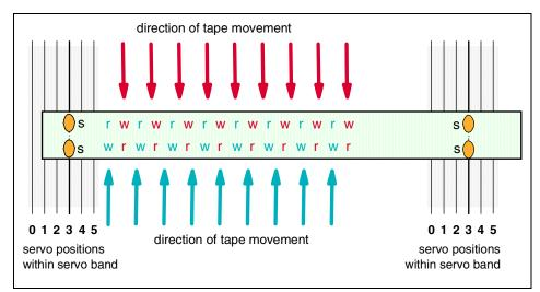
Figure 2-16 Allocation of read and write heads for forward and reverse wrap
