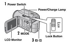
Set the appropriate operation mode according to your preference using the power and **MODE** switches and  $( \square / \square )$  button.
