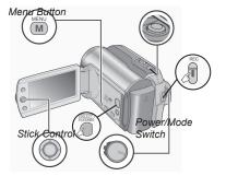
The movie camera icon represents recording video. The camera icon represents recording stills. The lamp will illuminate next to the icon for the present camera mode. Press the switch down to change recording modes.
