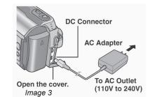
The battery will take 90 minutes to full charge. The lamp will blink indicating the battery is in the charging process. The lamp will turn of when the battery is completely charged.
