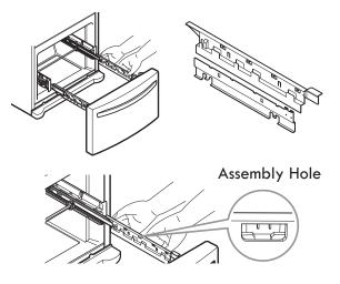
**NOTE:** Make sure that the left and right rail covers are attached to the correct rails. See picture below.
