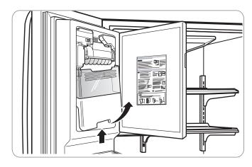
**3.** To reinstall the in-door ice bin, slightly slant the bin during replacement to avoid contact with the icemaker.
