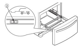
Grasp the drawer on each side and pull it up to separate it from the rails.
