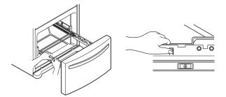
Remove the screws 2 of the rail on both sides.
