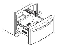
Press the tabs on each of the rail covers and lift them up to separate from the rail assembly.
