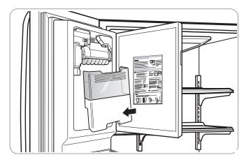
**4.** Avoid touching the ice-detecting sensor when replacing the ice bin. See the label on the ice compartment door for details.
