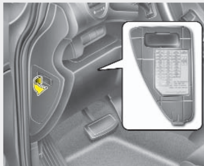
Inner fuse panel
