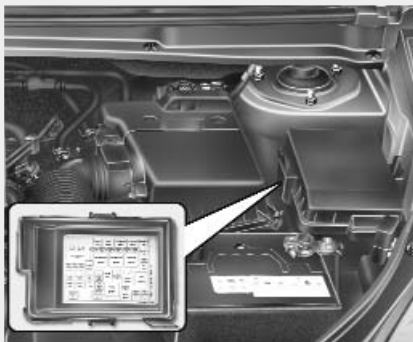
Engine compartment fuse panel
