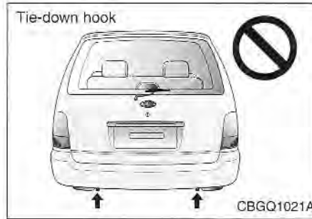
Tie-down Hook (for flatbed towing)
