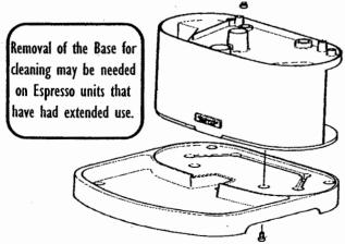
Remove the (6) Allen Bolts that hold the base to the Cabinet Main Body and clean the soiled surfaces with a warm soap and water solution.
