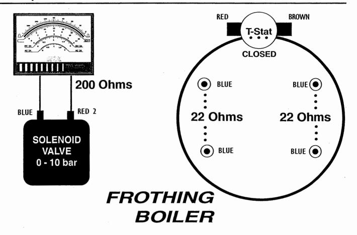
WIRE COLOR is denoted for the terminals that are on the device.
