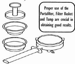
Either the small "One Shot" or large "Two Shot" Filter Basket shown above can be inserted into the Portafilter, depending on the amount of espresso the customer wants to brew.
