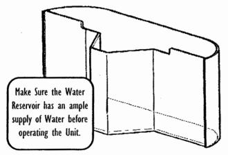
Each 1/2" of water level in the reservoir is (1) Cup of Water. Always keep water in the reservoir!
