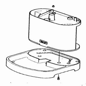
The Base Assembly and Cabinet Body shown on the left should be removed from the Cabinet Plate so the Technician will have access to the Core Components. These two items will normally require cleaning with a mild Soap Solution before reassembly. Be sure to replace any fastener that is oxidized or severely soiled.
