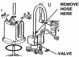
The Black Hose (Pipe SL) from the Espresso Boiler Valve (1- 10 bar) routes pressure through a hole in the Cabinet Body to the Drip Tray. When removing the Cabinet Body loosen the Spring Clip that connects the Hose to the Valve first. This will free the Cabinet Body for removal.
