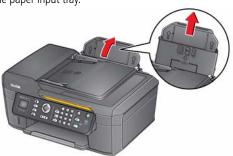
**2** Pull out the paper output tray and the extender until they are fully extended.
