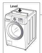
Check the leveling of the washer with a Level and check that the washer is stable.
