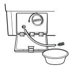
If SERVICE is needed during check, remove the remaining water by pulling out the hose cap.
