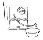
If SVC is needed during check, remove the remaining water by pulling out the hose cap.
