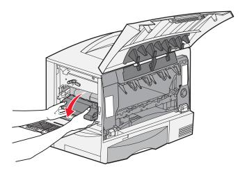
c Slide the image transfer unit out and place it on a clean, flat surface.
