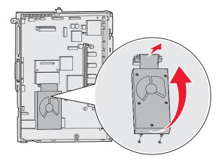
4 Gently pull the ribbon cable connector out of the connector on the system board.
