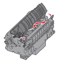
6 Lift up the fuser roller cover and remove the jam.
