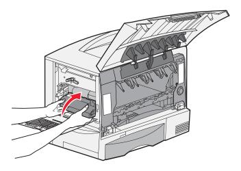
**c** Lower the lever to lock the image transfer unit into place.
