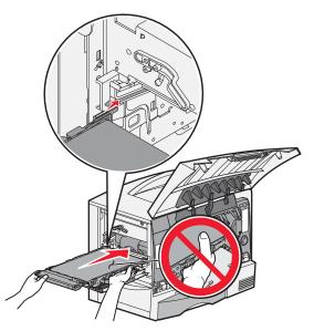
**b** Rotate the handle up, and push gently to lock the unit in place.
