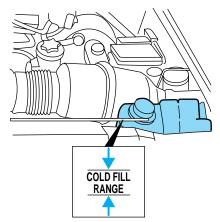
If the engine coolant has not been checked at the recommended interval, the engine coolant reservoir may become empty. If this occurs, add engine coolant to the reservoir. For more information on engine coolant maintenance, refer to *Adding engine coolant* in this chapter.
