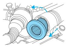
5. Replace the two halves of the air filter housing and secure the clamp.
