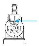
until the "0" mark on the yellow dial lines up with the reference mark on the marker (as shown) when viewed directly from above.
