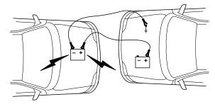
4. Make the final connection of the negative (-) cable to an exposed metal part of the stalled vehicle's engine, away from the battery and the carburetor.
