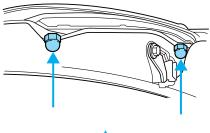
2. Carefully pull the lamp assembly outward to expose the electrical connector.
