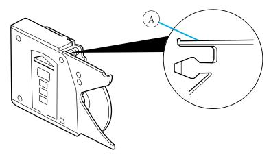
If you pull too hard on the disc holder, the disc holder may come completely out of the magazine. If this happens, reinsert the disc holder back into the magazine while pressing on the lever (A).
