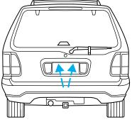
Do not leave the liftgate or liftgate glass open while driving. Doing so could cause serious damage to the liftgate and its components as well as allowing carbon monoxide to enter the vehicle.
