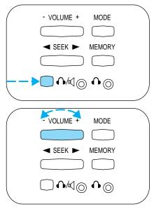
From the rear seat controls, volume control can be set no higher than the current radio setting unless the speakers are turned off. Refer to *Turning speakers on and off.*
