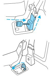
3. Use the black plastic clip (located just above the detachable anchor) to stow the loose seat belt.
