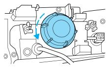
6. Release clip and disconnect the electrical connector from the bulb.
