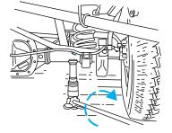
To lessen the risk of personal injury, do not put any part of your body under the vehicle while changing a tire. Do not start the engine when your vehicle is on the jack. The jack is only meant for changing the tire.
