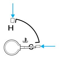
This gauge indicates the temperature of the engine coolant, not the coolant level. If the coolant is not at its proper level the gauge indication will not be accurate. If the gauge enters the red section, the oil pressure/engine coolant and *Check Engine/Service Engine Soon* indicators illuminate, refer to *What you should know about fail-safe cooling* in the *Maintenance and care chapter*.
