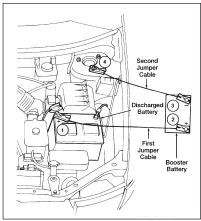
Sequence for connecting jumper cables
