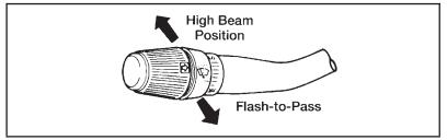
High beam and flash-to-pass operation
