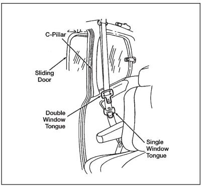
The auxiliary safety retraint system for the second row bench seat
