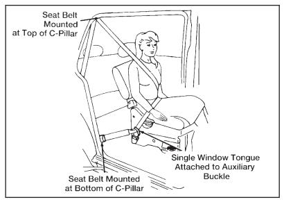
The auxiliary safety restraint system fastened
