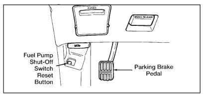
Fuel pump shut-off switch reset button location
