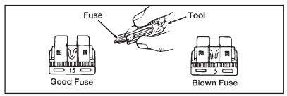
Fuse puller tool and fuse
