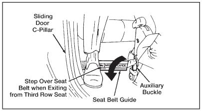
Exiting a vehicle with the auxiliary safety restraint system
