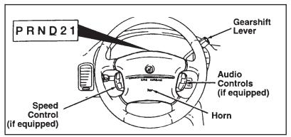
The steering column gearshift lever positions
