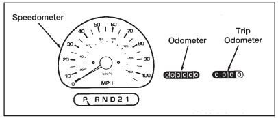
Speedometer, odometer and trip odometer
