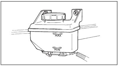
Brake fluid master cylinder reservoir
