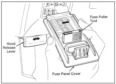
The instrument panel fuse panel
