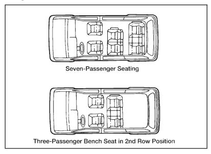
NOTE: Do not try to remove the three-passenger sliding seat. Removal of the third seat may negatively affect its ability to slide properly.
