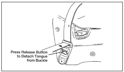
Unfastening the auxiliary safety restraint system
