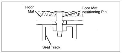
Floor mat positioning pin placement
