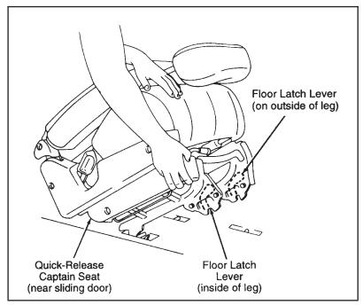
Removing the quick-release bucket seat
