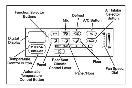
The ATC maintains the temperature you select and automatically controls the airflow for your comfort. It also allows you to override the automatic operation of airflow and fan speed with manual function selector buttons and the fan speed dial.
