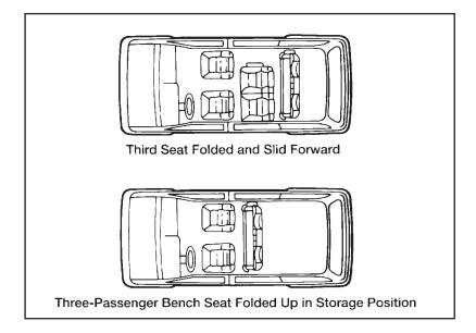
With the second row seat(s) removed, the three-passenger bench seat can be moved all the way forward, just behind the front seats for more room in the cargo area.
