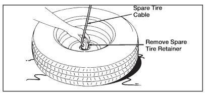
Removing the spare tire retainer
