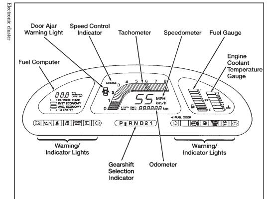
The electronic cluster has all of the same warning lights as the mechanical cluster, however, some of the gauges will be electronic instead of analog. In addition, the electronic cluster has a fuel computer which displays fuel economy, distance to empty and outside air temperature.
