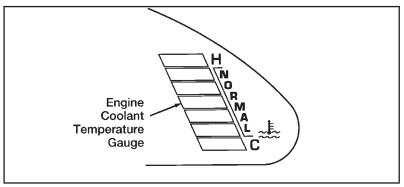
Engine coolant temperature gauge
