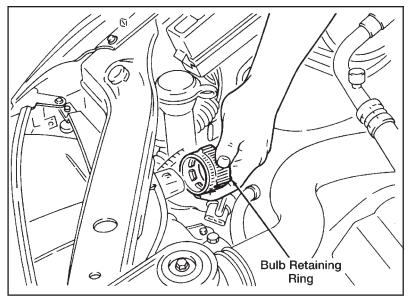
Removing the headlamp bulb retaining ring
