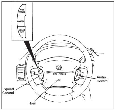
Speed control buttons on the steering wheel
