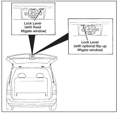
Locking the liftgate using the lock lever
