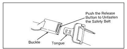
Unfastening the combination lap and shoulder belts — front and rear outboard seating positions
