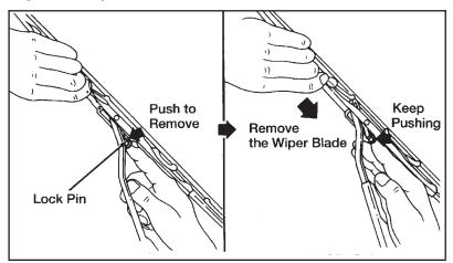
Replacing the wiper blades
