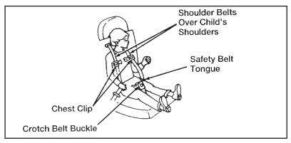
4. Place the left shoulder belt harness over the child's left shoulder. Insert the left shoulder harness tongue into the left side of the belt buckle. Confirm that the left shoulder harness tongue indicator is green.
