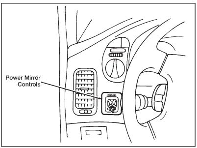
Dual electric remote controlled mirrors switch
