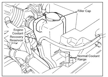
Engine coolant recovery reservoir
