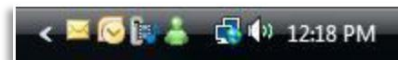
Figure 10. Each icon represents at least one running process and sometimes many more
