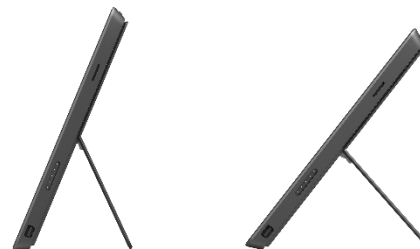
Surface Pro 2: Dual position kickstand
