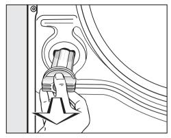
Withdraw the two struts together with the support plate.
