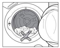
Close the drum door. To prevent damage make sure that there are no clothes caught between the drum door and seal.
