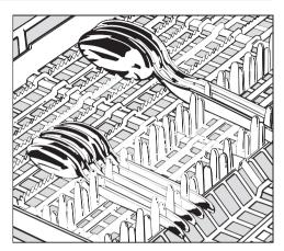
Spoon heads should be placed in contact with at least one of the serrated retainers of the cutlery tray to ensure that water runs off freely.
