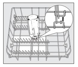
The bottle holder e.g. for milk or baby bottles, can be inserted into the bottom basket in more than one place. Position in any area marked white in the illustration. Do not place the insert in the corners of the lower basket, water cannot properly cover bottles in these areas. Additional inserts for the upper and lower baskets may be purchased from your Miele dealer or the Miele Technical Service Department.
