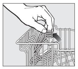
Raise the rack to make room for tall glasses. Lower it to double stack smaller pieces.
