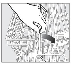
To allow water to run off the bottom of coffee mugs, place slanted on top of the coffee bar. The bar can also be used to separate two rows of glasses. To stack wide items, flip the bar to the right.
