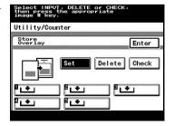
If a button is pressed where no image is stored, the size of the stored image appears on the button to indicate that an image has been stored.
