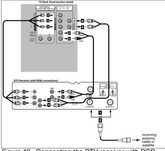
Figure 13. Connecting the DTV receiver with RGB video connections.
