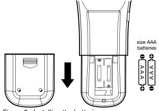
Figure 2. Installing the batteries.
