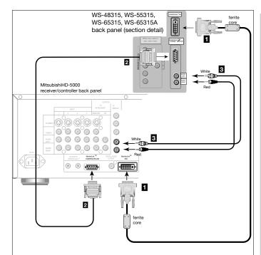
Figure 14. Connecting MonitorLink
