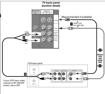
Figure 6. Connecting the VCR Audio/Video.
