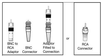
Figure 11. DTV connectors and adaptors.
