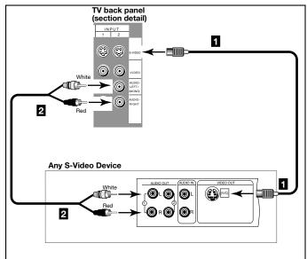
Figure 10. Connecting an S-Video Device.
