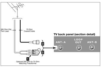
Figure 2. Connecting twin lead antenna, coaxial lead antenna, or wall outlet cable.
