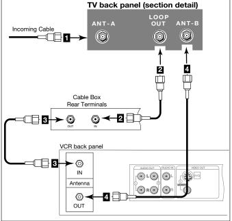
Figure 5. Connecting the VCR with cable box.
