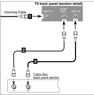
Figure 3. Connecting the cable box.
