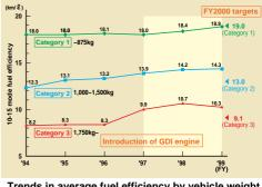
Trends in average fuel efficiency by vehicle weight category (gasoline-powered passenger cars)
