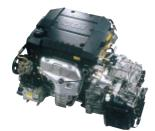
GDI turbo engines take full advantage of the outstanding anti-knocking properties of GDI engines, and at the same time offer better response and fuel efficiency than conventional turbo engines. A GDI turbo engine was adopted for the Pajero io in July 2000, which not only cleared the 2000 exhaust controls, but was also the first turbo car to pass the 2010 fuel efficiency standards.
