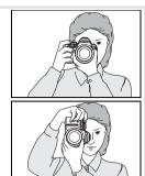
**4.2** Smoothly press the shutter-release button the rest of the way down to release the shutter and record the photograph. The access lamp next to the memory card slot cover will light. Do not eject the memory card or remove or disconnect the power source until the lamp has gone out and recording is complete.
