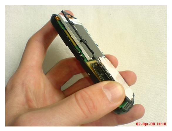
• Lift the PCB from left to right at the top of the phone. Be careful and do not remove it completely as it's held in place at the bottom of the phone by the ringer. You just need to lift it out enough to access the connector from the LCD screen, circled below. This connects
