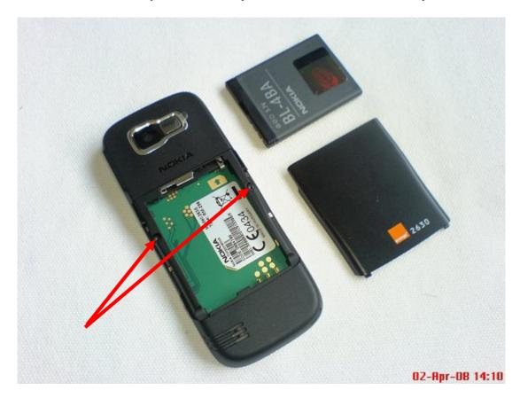
• The front cover can be removed by unclipping it starting at the middle of the cover (where you just removed the two screws).
