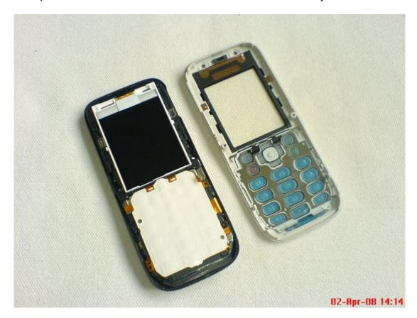
• The LCD is held in place by a plastic frame which is held to the PCB with clips around its edge. Unclip the frame from left to right, like below. Don't remove it completely, but leave it attached on the right side.
