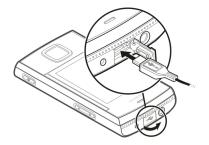
Open the cover of the USB connector, and connect the USB cable to the device.
