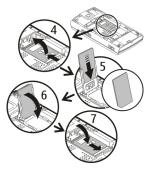
3 Line up the battery contacts, and insert the battery. Replace the back cover.
