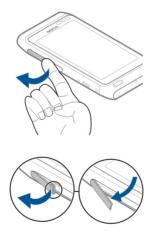
2 Make sure the contact area of the memory card is facing down, and insert the card. Push the card in, until it locks into place.
