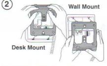
Attach the wedge-shaped base in desk mount or wall mount position.
