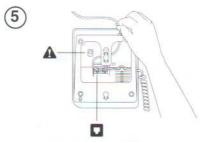
Connect the line cord. Connect the power adapter.
