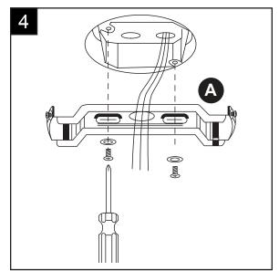
**Note**: Remove the preassembled short mounting screws (CC) from the mounting bracket (A) and motor assembly (B) before continuing to the next step.
