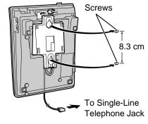
Tuck the telephone line cord inside the wall mounting adaptor, and push it in the direction of the arrow.
