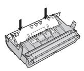
**9** Turn the two green levers (①) on the toner cartridge firmly.
