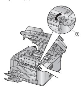
2. Remove the jammed paper (1) carefully by pulling it upwards.
