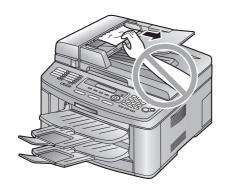
1 Hold the ADF cover firmly and lift it to open the upper part (①) of the ADF cover.
