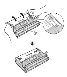
**6** Remove the used cartridge (1) from the drum unit (2).
