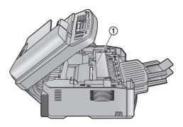
**5** Reinstall the drum and toner unit (①) by holding the tabs.
