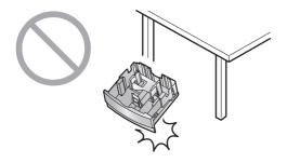
Hold the paper input tray with both hands when removing or installing. The input tray weights approximately 2 kg (4.4 lb.) when the recording paper is fully installed.
