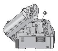
8 Install the drum and toner unit (1) by holding the tabs.
