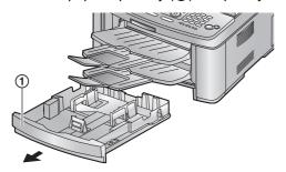
**2** Pinch the front side of the recording paper guide (①), then slide it to match the paper size mark.
