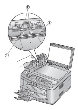
5 Close the ADF cover (①), then hold the document cover (②) while cleaning the white plate (③) and the scanner glass (④).
