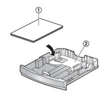
Make sure that the recording paper guides (1) are at the paper size mark and the recording paper is under the paper limit mark (2). The paper should not be over the snubbers (3).
