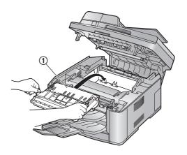
Make sure that the triangles (②) match to install the drum and toner unit correctly.
