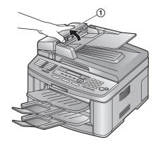
**3** Press the ADF cover release button (1) and open the middle part (2) of the ADF cover.
