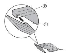
2. Slide the other tab (①) into the right hole (②) of the extender from below until it clicks into place.
