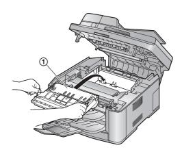
• Make sure that the triangles (2) match to install the drum and toner unit correctly.
