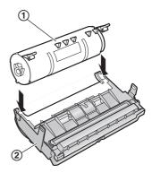
**4** Firmly press down the toner cartridge to snap into position.
