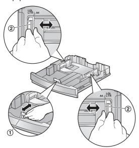
Before loading a stack of paper, fan the paper to prevent paper jams.
