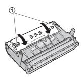
**10** Make sure that the triangles (①) match to install the toner cartridge correctly.
