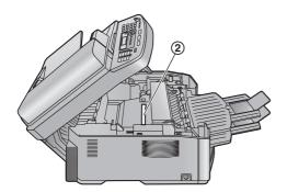
**11** Install the drum and toner unit (①) by holding the tabs.
