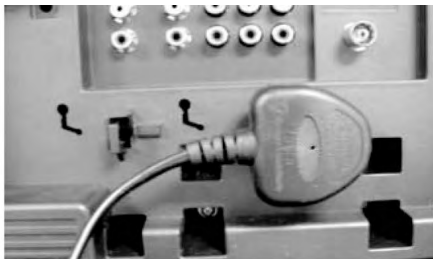
Fix AC cord into the 3-pin plug hole at the back cover
