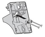
Tuck the telephone line cord inside the wall mounting adaptor (♠). Connect the AC adaptor cord and telephone line cord (♠).
