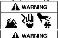
If you perform any maintenance on the engine, first disconnect the spark plug wire from the spark plug, and disconnect the battery at the negative terminal (electric starter engines only) to prevent unintentional sparking. Unintentional sparking can result in fire or electric shock. Unintentional start-up can result in entanglement, traumatic amputation or laceration. Use only correct tools.
