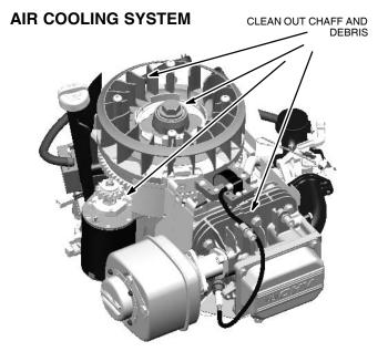
Debris may clog the engine's air cooling system. Remove blower housing and clean area shown to prevent overheating and engine damage.
