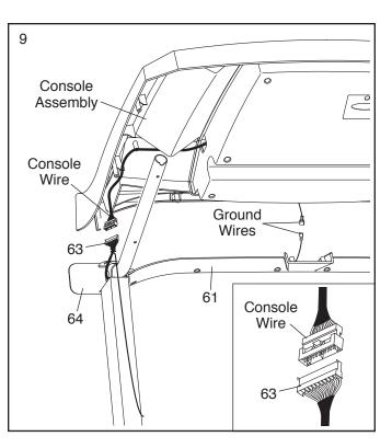
Insert the wires into the Right Handrail (64) through the indicated hole as you set the console assembly on the Left and Right Uprights (66, 76). Make sure that no wires are pinched.
