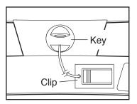
displays will light. **IMPORTANT: In an emergency**, the key can be pulled from the console, causing the walking belt to slow to a stop. Test the clip by carefully taking a few steps backward; if the key is not pulled from the console, adjust the position of the clip.
