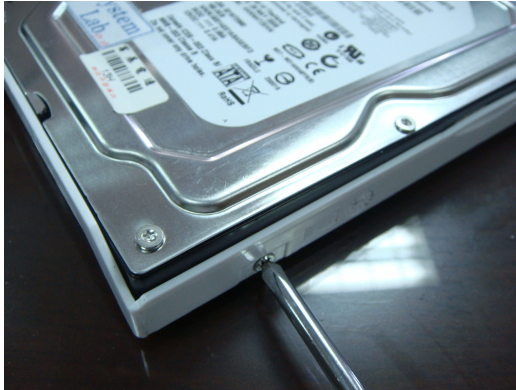
Figure 2. Remove the disk drive from the drive carrier
