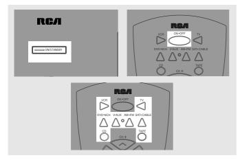
• Standby: when the receiver is on, press the **ON/STANDBY** button once to activate the standby mode.
