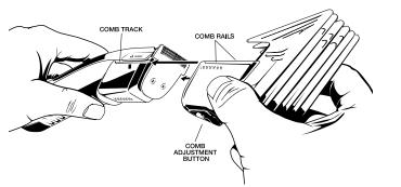
To attach comb to clipper, align both comb rails with the comb tracks on both sides of the clipper and slide into place. Once comb is secure you will hear a click sound, letting you know it is locked in. Ensure comb is properly secured by pushing down on comb, the comb should not slip. To adjust comb height press down on the comb adjustment button and slide up or down as necessary.
