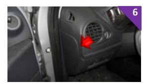
Using the plastic trim tools, unclip the panel located on the left side of the dashboard.
