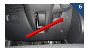
Run the cable under the steering wheel panel towards the radio housing, attaching with wire ties.
