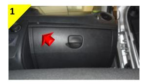
On the top side of the glove box, insert the cable into the hole.
