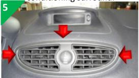
Using the plastic trim tools, unclip and remove the central air vent.
