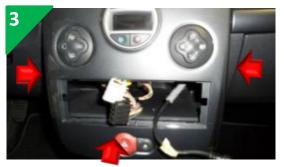
Using the plastic trim tools, unclip the car stereo and air conditioning surround.
