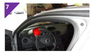
Remove the door seal on the driver's side.
