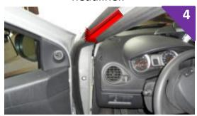
Run the cable along the driver's side windscreen support while replacing the door seal.
