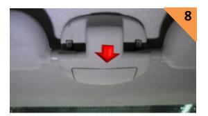
Using the plastic trim tools, unclip and open (without removing) the panel in between the two sun visors.
