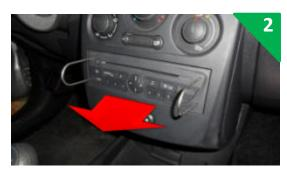
Carefully release the radio, without pulling it out completely, so that you can disconnect the connectors and the antenna. Then completely remove the radio.
