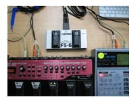
Using a dual TRS connecter & a couple of stereo "Y" cables I connected to the CLT ports 1,2 & 3,4 on both units.
