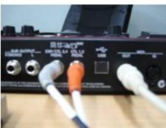
Once connected, you will need to assign the control function for each control port. I assigned Patch Decrease to CLT 1,2 & Patch Increase to CLT 3,4 on both units.
