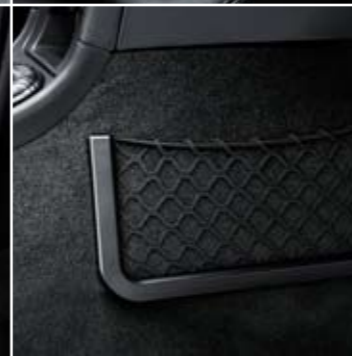
Net pocket – elastic net fitted on the passenger side of the centre console.
