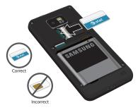
Note: If the card is not inserted correctly, the phone will not detect the SIM card. Re-orient the card back into the slot if the SIM is not detected.
