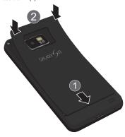
Press along the edge of the back cover (3) until you have a secure seal.
