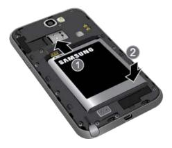
Replace the battery cover, making sure all the tabs are secure and there are no gaps around the cover.
