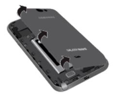
• Insert the battery, contacts end first, and gently press the battery into place.
