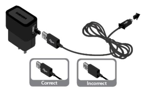
3. Plug the USB connector into the charger/accessory jack on the bottom of your phone.
