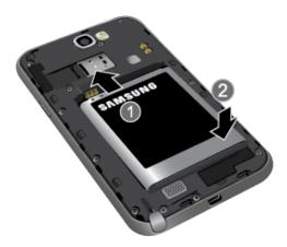
• Replace the battery compartment cover, making sure all the tabs are secure and there are no gaps around the cover.
