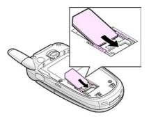
Note: When you need to remove the SIM card, slide it, as shown, and take it out of the socket.
