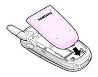
Press the battery until it clicks into place. Make sure that the battery is properly installed before switching the phone on.
