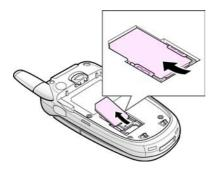
5. Place the battery so that the tabs on the end align with the slots at the bottom of the phone.
