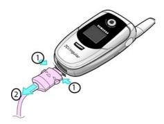
**Note:** You must unplug the adapter before you remove the battery from the phone during charging; otherwise, the phone could be damaged.
