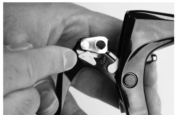
2. Align the mode switch with the position of the brake installed.
