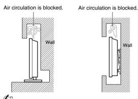
Inadequate air circulation can lead to overheating of the TV and may cause damage to your TV or cause a fire.
