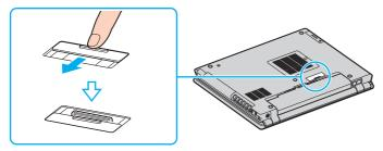
5 Slide the LOCK/UNLOCK switch on the multi function bay docking station to UNLOCK.
