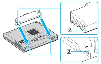
4 Rotate the battery in the direction of the arrow, and push the battery down into the compartment until it clicks into place.
