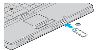
Be sure to hold the Memory Stick media with the arrow pointing in the correct direction as you insert it into the slot. To avoid damaging the computer or the Memory Stick media, do not force the Memory Stick media into the slot if it does not insert smoothly.
